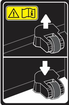
Caution: Always leave the pinch rollers in the upper positions when the cutter is not in use.
