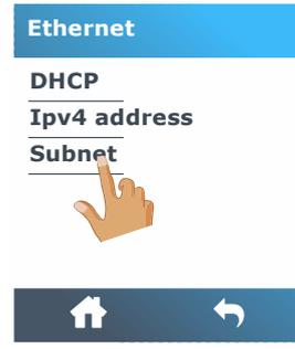
9. Set the address correctly. 10. Confirm by pressing
