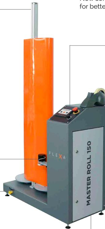
Made from powder coated sheet steel and anodized aluminium sections
