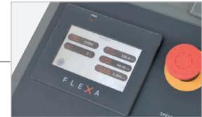
Touch screen display to select the rewinding parameters
