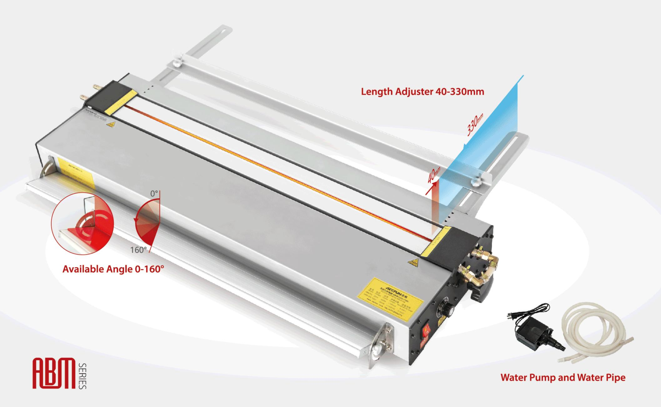
Acrylic bending machine is also called plastic plate bending machine, soften and bend the plastic plate by heating.
