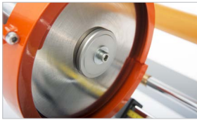
Dual chamfer blade (standard). Single chamfer blade (optional) for fabrics and narrow reels of 5 cm
