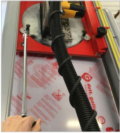
Comfortable handle for the vertical sliding of the cutting carriage
