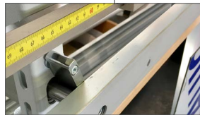
Depth adjustable intermediate support for cutting small size pieces
