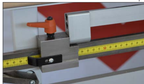
Reference bar mounted on a practical millimeter scale for fast and precise cuttings
